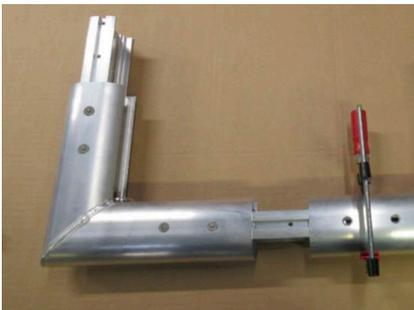
**Screw and tighten the screws in alternation crosswise!**
